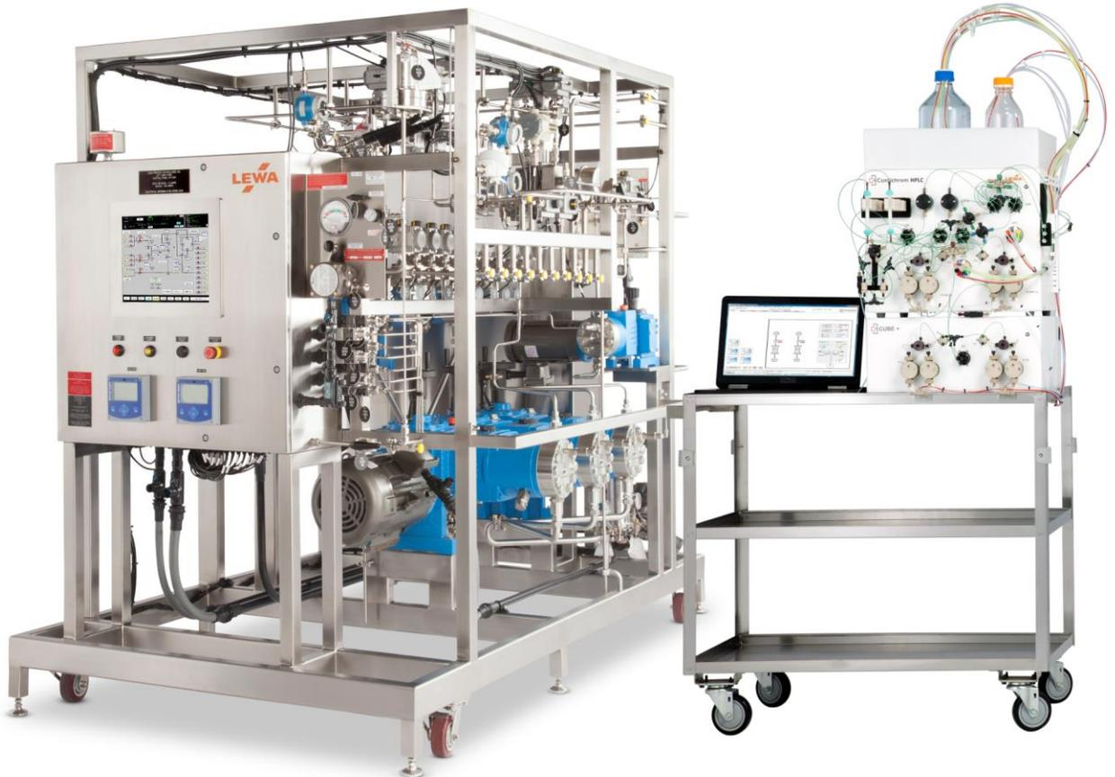
LEWA designed, automated and manufactured process scale HPLC
